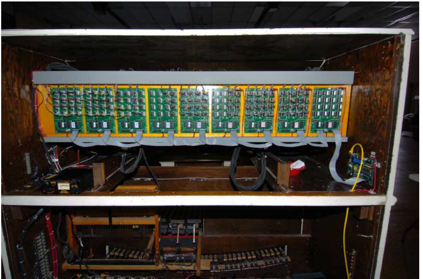
Rear view showing the various connections between the boards and organ components.
