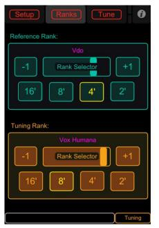
There are two ranks used by the remote tuner. The first rank is called the "Reference" rank and is typically the rank that other ranks are tuned against. The second rank is called the "Tuning" rank and is typically the rank that is being tuned. When tuning a rank against itself (usually the first rank being tuned), both ranks can be assigned to the same rank and typically are pitched one or two octaves apart for initial tuning.
