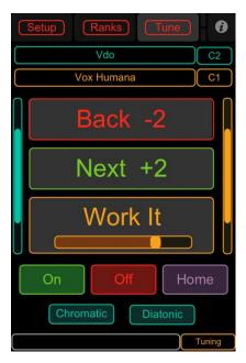
This is where the actual work is done. The top two lines show the rank names and current note being tuned. As with the previous rank selection page, the reference rank is shown in Blue and the tuning rank is shown in Orange.
